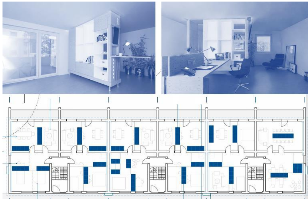
Fig. 10. Floor plan variations for the transformation of linear block typologies in the case study: adapting spaces to new domestic programs. M. Pelegrín, F. Pérez, D. Ercin, BIM Labor, 2023. Source: Preliminary report of the research project H&O?.
